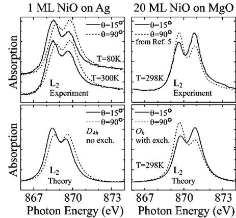
FIG. 3. Polarization dependence of the Ni  $L_2$  XAS of 1 ML NiO on Ag(100) covered by MgO(100). The 20 ML NiO on MgO spectra are taken from Ref. 5. The theoretical spectra for the 1 ML NiO are calculated in  $D_{4h}$  symmetry without exchange, and for the 20 ML in  $O_h$  with exchange.
