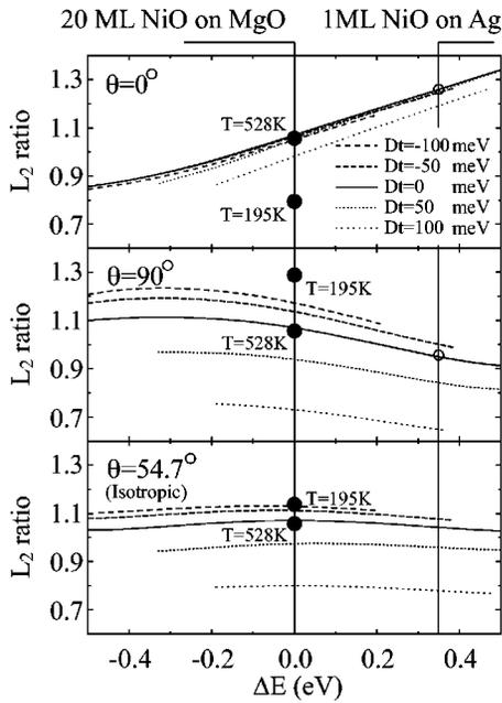
FIG. 5. Calculated ratio of the two peaks in the  $L_2$  edge as a function of  $\Delta E$ , which is the shift in energy of the  $L_3$  main peak in going from grazing ( $\theta=0^\circ$ ) to normal ( $\theta=90^\circ$ ) incidence of the linearly polarized light. The  $L_2$  ratio is calculated for  $\theta=90^\circ$ ,  $\theta=0^\circ$ , and for the isotropic spectrum.
