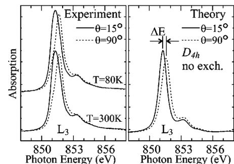
FIG. 4. Experimental and theoretical polarization dependence of the Ni  $L_3$ -XAS of a 1 ML NiO(100) on Ag(100) covered with MgO(100). The theoretical spectra are calculated in  $D_{4h}$  symmetry without exchange.
