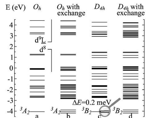
FIG. 1. Energy level diagram for  $\text{Ni}^{2+}$  ( $3d^8$ ) in: (a)  $O_h$  symmetry with  $pd\sigma = -1.29$  and  $10Dq = 0.85$  eV; (b)  $O_h$  symmetry with additional exchange field of 0.16 eV; (c)  $D_{4h}$  symmetry with  $pd\sigma = -1.29$ ,  $10Dq = 0.85$ , and  $Ds = 0.12$  eV; (d)  $D_{4h}$  symmetry with additional exchange. The  $3d$  spin-orbit interaction is included, but the states are labeled as if the spin-orbit interaction was not present.
