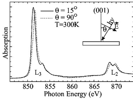
FIG. 2. Experimental polarization dependent Ni  $L_{2,3}$  XAS of 1 ML NiO(100) on Ag(100) covered with MgO(100).  $\theta$  is the angle between the light polarization vector and the (001) surface normal ( $\theta=90^\circ$  means normal light incidence).
