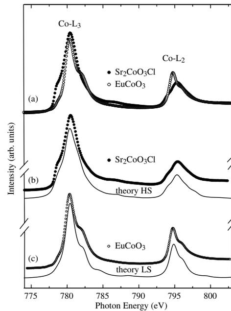
FIG. 2. (a) Co  $L_{2,3}$  XAS spectra of  $\text{Sr}_2\text{CoO}_3\text{Cl}$  (●) and  $\text{EuCoO}_3$  (○). (b) Comparison between the  $\text{Sr}_2\text{CoO}_3\text{Cl}$  spectrum (●) and a theoretical simulation for a high-spin (HS)  $\text{CoO}_5$  pyramidal cluster (solid line). (c) Comparison between the  $\text{EuCoO}_3$  spectrum (○) and a theoretical simulation for a low-spin (LS)  $\text{CoO}_6$  octahedral cluster (solid line).
