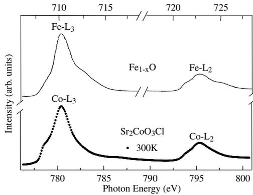
FIG. 1. Co  $L_{2,3}$  XAS spectrum of  $\text{Sr}_2\text{CoO}_3\text{Cl}$  measured at 300 K (●) and Fe- $L_{2,3}$  XAS spectrum of  $\text{Fe}_{1-x}\text{O}$  ( $x \leq 0.05$ ) reproduced from Ref. [32] (solid line).
