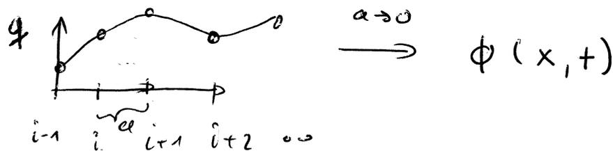
$$\partial_t^2 q_i = c^2 ([q_{i+1} - q_i] - [q_i - q_{i-1}]) / a^2 \quad (1.1)$$
