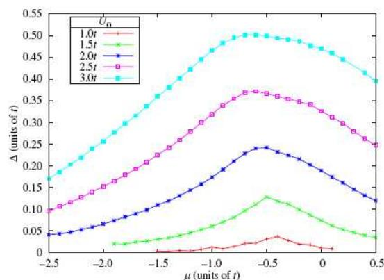
**Figure 15.** Magnitude of the superconducting order parameter  $\Delta$  as calculated via the interaction flow procedure for varying interaction strength  $U_0$  and chemical potential  $\mu$ ,  $t' = -0.1t$ .
