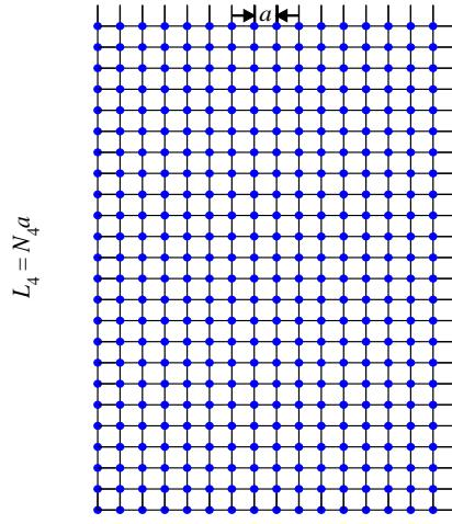
$$\begin{aligned} x &\longrightarrow x_n \\ \phi(x) &\longrightarrow \phi_n \equiv \phi(x_n) \\ \partial_\mu \phi(x) &\longrightarrow \frac{1}{a}(\phi_{n+\hat{\mu}} - \phi_n) \end{aligned}$$
