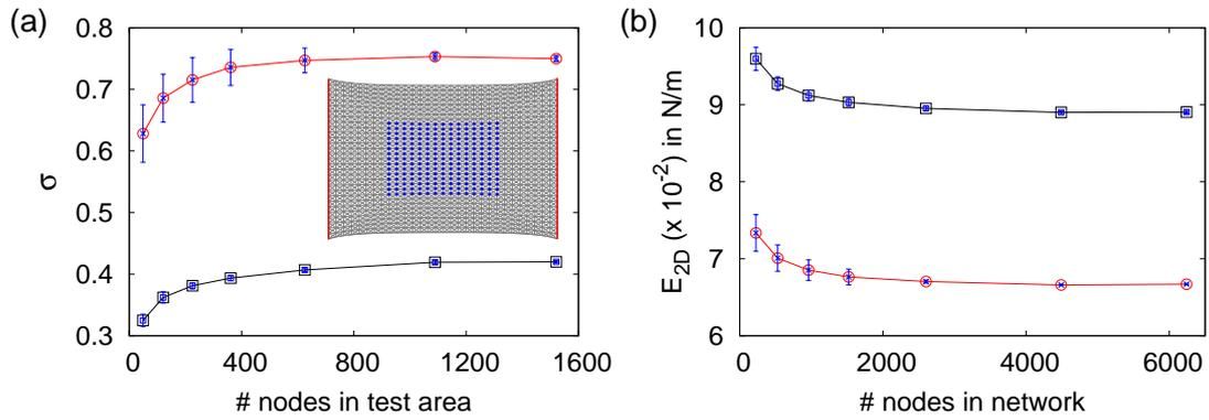
FIG. 1: (a) Effective Poisson ratio  $\sigma$  and (b) effective two-dimensional Young modulus  $E_{2D}$  for the reinforced square network as a function of the number of nodes in the test region. In both cases, red and blue curves are for networks without and with prestrain, respectively. Thus prestrain decreases  $\sigma$  and increases  $E_{2D}$ . The inset shows the deformed network and the test region in the middle.
