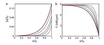
FIG. 2 (color online). Plot of (a) displacement |u| and (b) stress *F* within the cell layer for the stripe geometry with  $P_0 = 0.7$ ,  $E_c = 10$  kPa,  $h = 1 \ \mu$ m,  $\nu = 0.45$ , and  $\gamma = 5, 6, 8, 10, 15$  [from top to bottom in (a) and from bottom to top in (b)].
