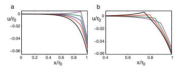
FIG. 3 (color online). Plot of displacement u in a disc with contractile rim for (a)  $P_0/P_1 = 0.1$ , 0.3, 0.5, 0.7, 1 with  $r_1/r_0 = 0.9$  (from top to bottom), (b)  $r_1/r_0 = 0.75$ , 0.8, 0.85, 0.9, with  $P_0/P_1 = 0.5$  (from top to bottom). In both plots  $\gamma = 8$ ,  $P_1 = 0.7$ ,  $\nu = 0.45$ .
