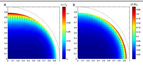
FIG. 4 (color online). Plot of (a) displacement |u|, arrows indicate displacement directions and magnitude, (b) traction force  $f/Kr_0$  exerted on pillars. In both plots  $\gamma = 5$ ,  $P_0 = 0.8$ , and  $\nu = 0.45$ ,  $\epsilon = 3$  (major axis in x direction), the dotted black line indicates the initial shape of the layer.
