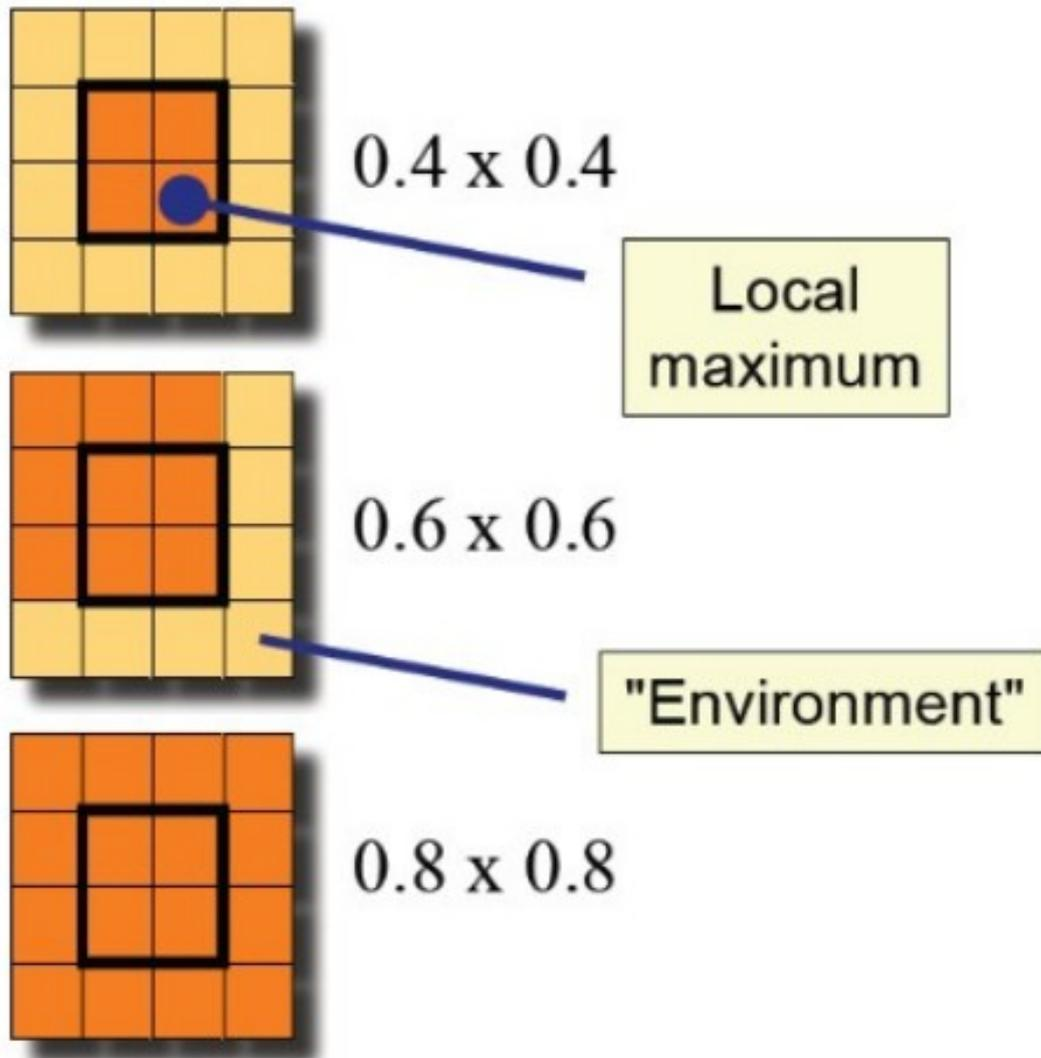
**Jet triggers can have varying sliding window sizes**
