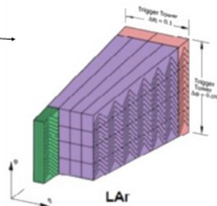
$\sim$  250k calorimeter cells summed on detector to 7168 projective trigger towers
