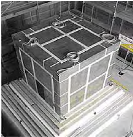
The 7-layered magnetically shielded room (residual field < 2 nT)
