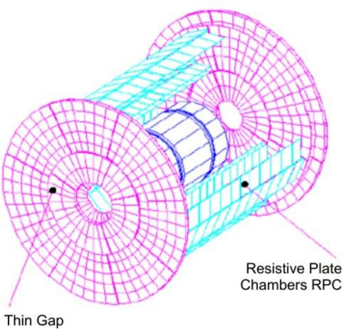
Thin Gap Chambers TGC Dedicated trigger chambers with good timing resolution, divided into 208 sectors
