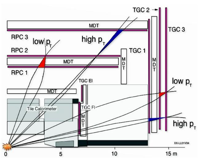
Level-1 Muon Trigger requires coincident hits in different RPC (barrel) or TGC (endcap) layers
