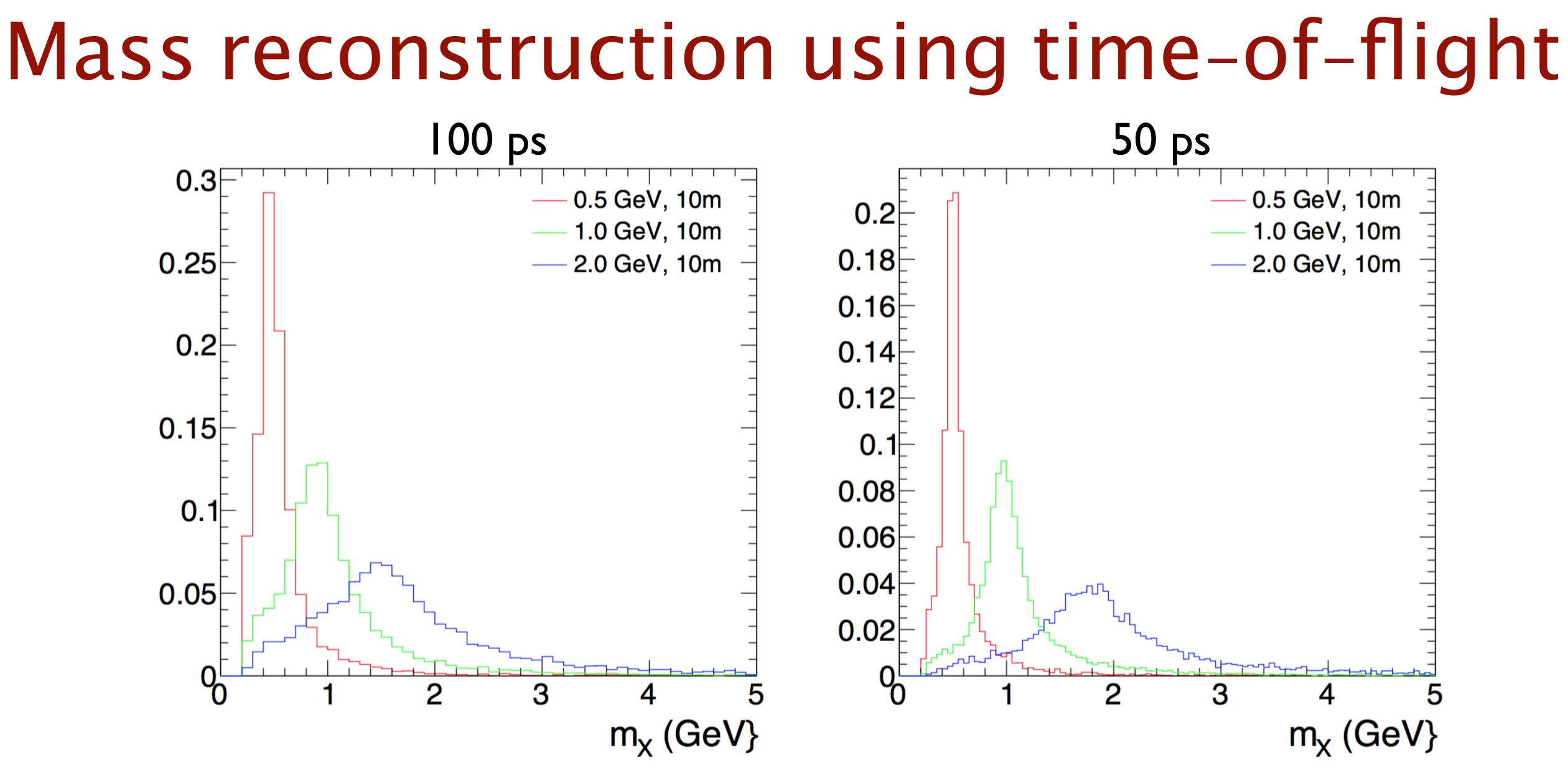
Now assume 100/50 ps time resolution (per hit) in the tracking stations. The  $B \rightarrow KX$  signals are actually slow enough that we can reconstruct the X mass...
