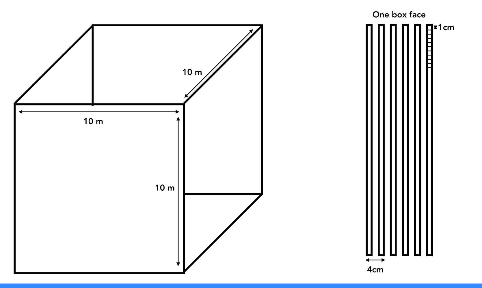
10x10x10 metre box, with 6 RPC layers on each box face. Assume 1 cm granularity for the RPCs, and possibility of timing information (explored later in talk). Add 5 other triplets of RPC layers equally spaced in box to minimize the distance to the first measured point for the decay vertex determination.
