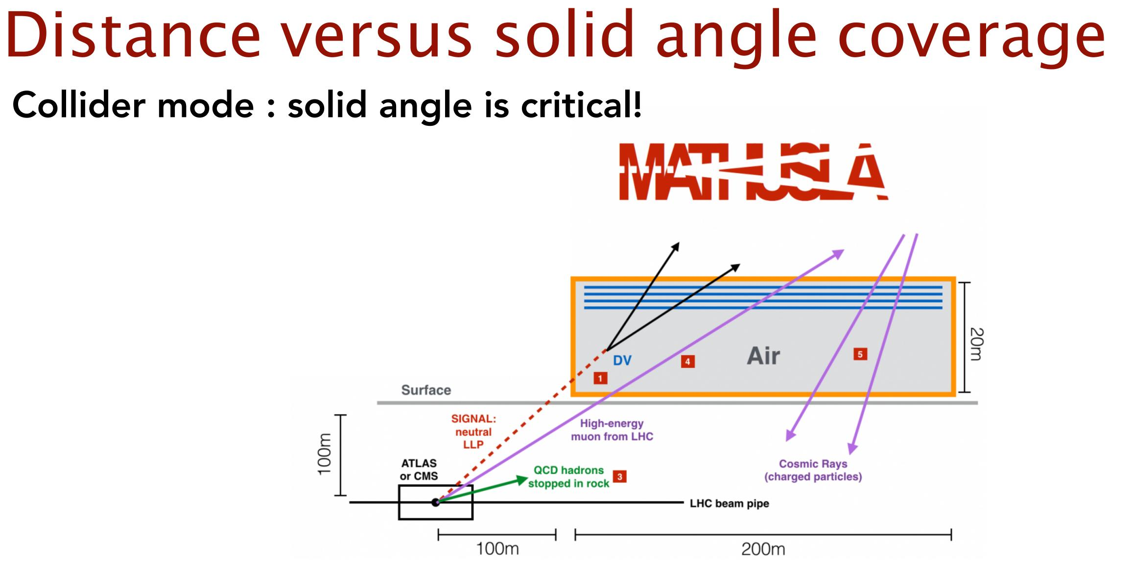
Uncollimated production means that unless you go forward like FASER, the size of your detector goes quadratically with the distance from collision point. Hence MATHUSLA's 200x200 m<sup>2</sup>...
