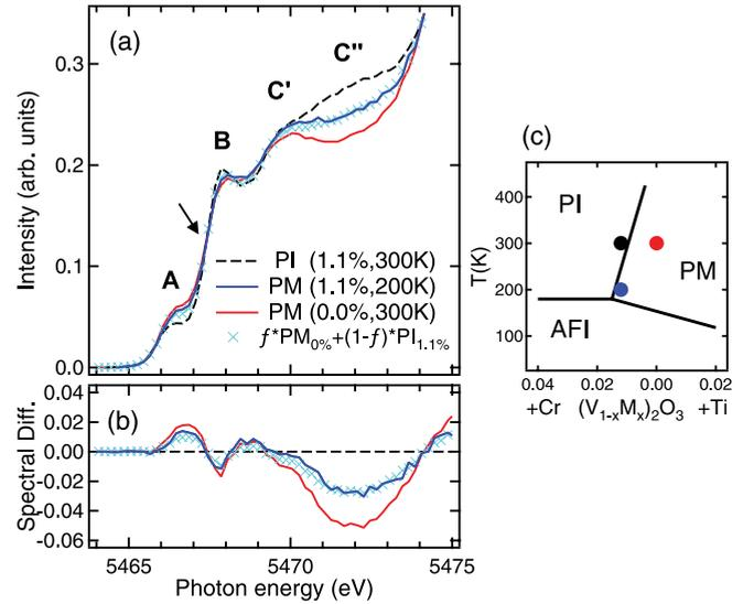
FIG. 7. (Color online)  $V K$ -pre-edge x-ray absorption spectra for a  $(V_{1-x}Cr_x)_2O_3$  powder sample as a function of temperature and doping level in PFY mode ( $x = 0, 0.011$  and  $T = 200$  and  $300$  K); crosses represent a linear combination of the room-temperature spectra ( $PM_{0\%}$  and  $PI_{1.1\%}$ ) for a value of  $f = 0.54$ ; (b) PI-PM spectral differences; (c) corresponding points in the phase diagram.
