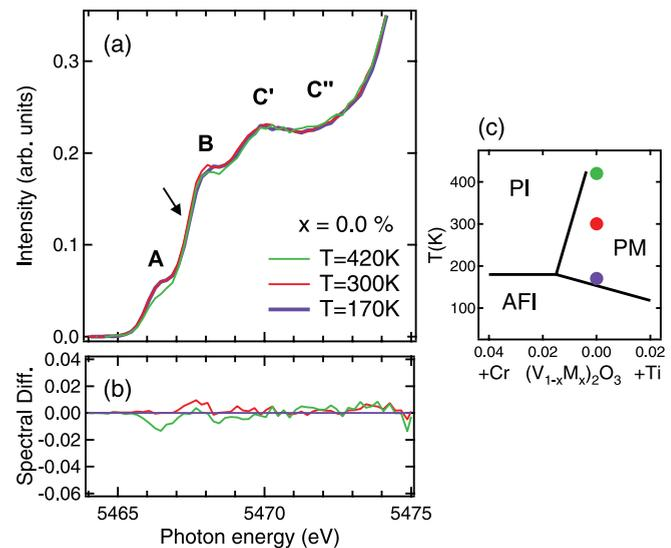
FIG. 6. (Color online) V  $K$ -pre-edge x-ray absorption spectra for a  $V_2O_3$  (PM) powder sample as a function of temperature in PFY mode ( $T = 170, 300$ , and  $420$  K); (b) spectral differences, with respect to the low-temperature spectra; (c) corresponding points in the phase diagram.
