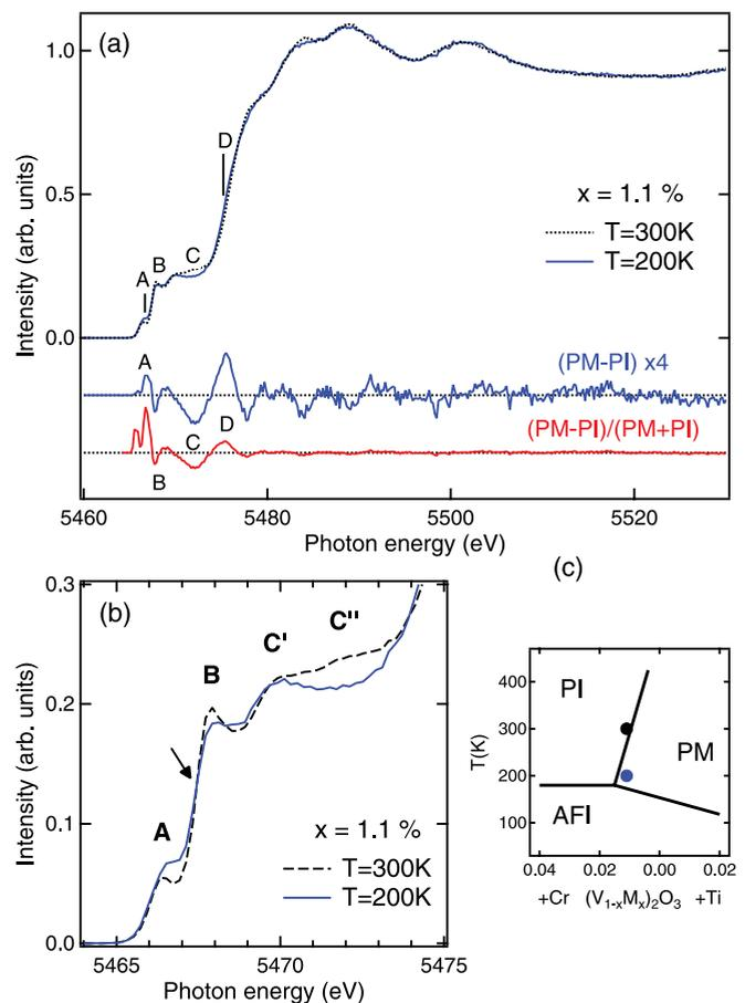
FIG. 4. (Color online) (a)  $V K$ -edge x-ray absorption spectra in a  $(\text{V}_{0.989}\text{Cr}_{0.011})_2\text{O}_3$  powder sample measured as a function of temperature in the PI (300 K, dashed line) and PM (200 K, solid line) phases in PFY mode; below, the blue (dark grey) curve shows the absolute spectral difference, while the red (light grey) curve represents the relative spectral difference; (b) pre-edge region; (c) corresponding points in the phase diagram.
