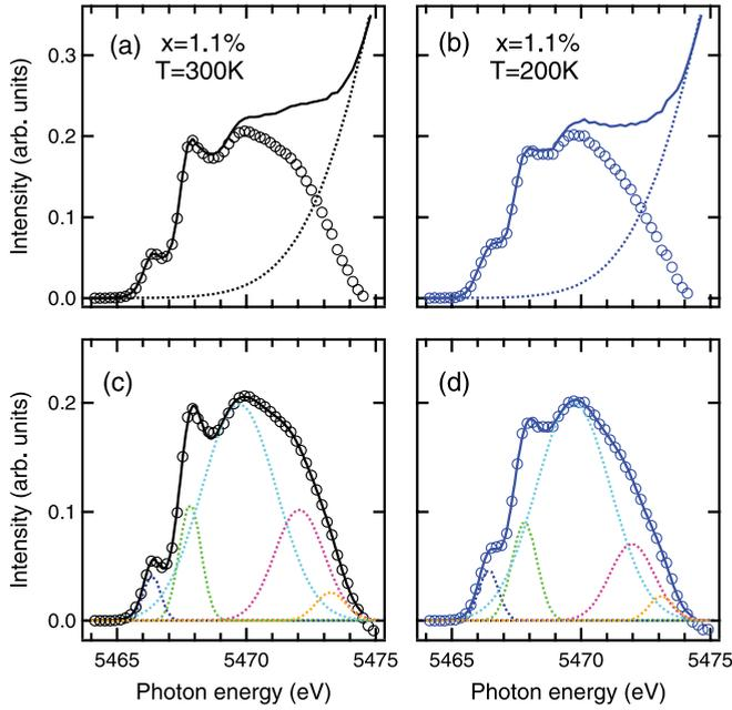
FIG. 10. (Color online) Illustration of the pre-edge fitting procedure for the data obtained on the  $(V_{0.989}Cr_{0.011})_2O_3$  sample across the temperature-induced MIT: after subtraction of the dipolar tails (dotted lines, top panels), the remaining features (circles) are fitted using five Gaussian functions (dotted lines, bottom panels). The maxima of the first two Gaussians corresponding to the peaks A and B are used to display the  $I(A)/I(B)$  evolution in Figs. 9(d)–9(f).
