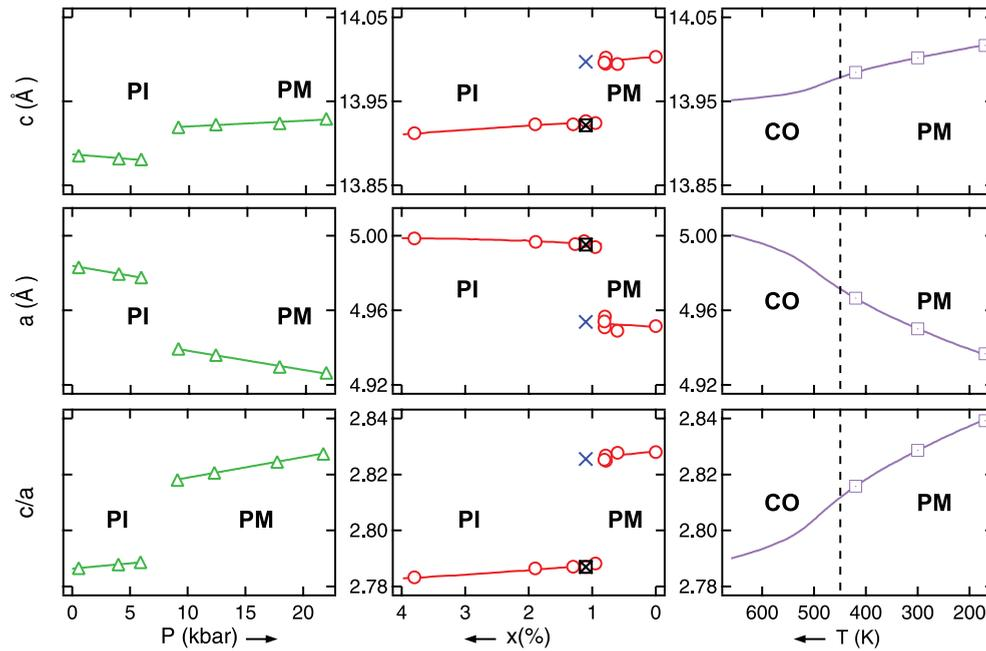
FIG. 11. (Color online) Lattice parameters as a function of pressure ( $x = 2.8\%$ , green triangles; the pressure scale refers to the  $x = 2.8\%$  doping), doping level (red circles, from Ref. 1), and temperature ( $x = 0\%$ , purple square, from Ref. 1). On the middle panel, we also present the lattice parameters measured in a  $(V_{0.989}Cr_{0.011})_2O_3$  sample across the temperature-induced MIT in the PI (300K, black crossed square) and PM phases (200K, blue cross).
