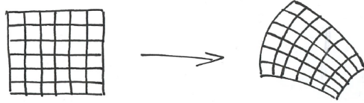
Figure 11: Illustration of a conformal mapping of a given field configuration to a new one.
