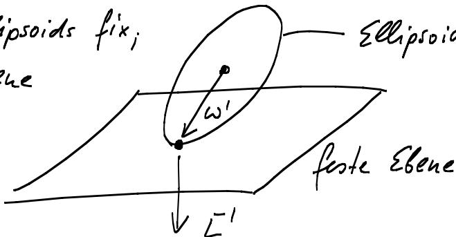
$$\text{Ellipsoid } E = \frac{1}{2} I_{ij}' \omega_i' \omega_j'$$
