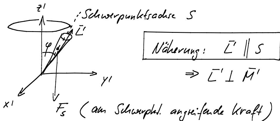
$$\dot{\bar{L}'} = \bar{M}' \xrightarrow{\bar{L}' \perp \bar{M}} |\bar{L}'| = \text{const.}$$
