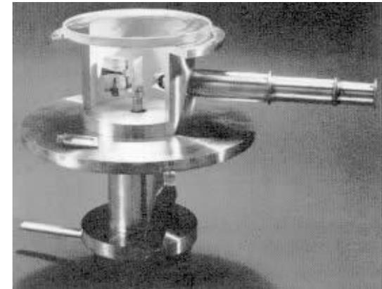
This apparatus was described in a 1913 paper by Geiger and Marsden. It was designed to accurately measure the scattering pattern of the alpha particles produced by the metal foil (F). The microscope (M) and screen (S) were affixed to a rotating cylinder and could be moved a full circle around the foil so that they could count scintillations from every angle.
