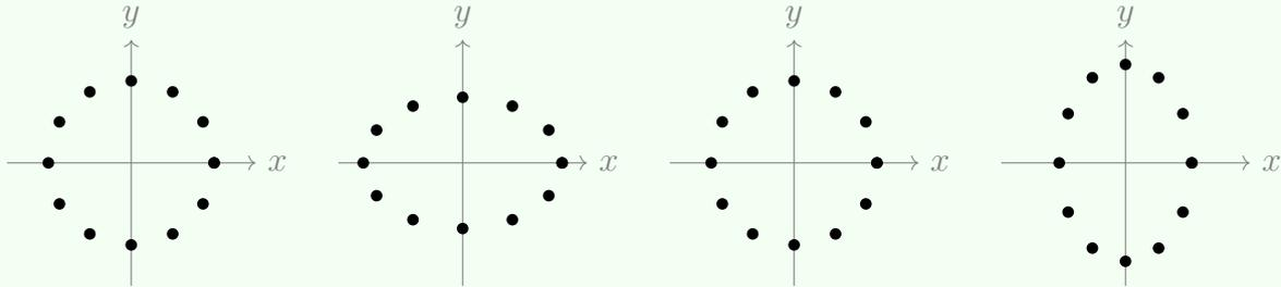
**Figure 2.1:** The effect a  $+$ -polarized gravitational wave propagating in  $z$ -direction has on a ring of freely falling particles placed in the  $x - y$ -plane. Each plot displays a snapshot in time.
